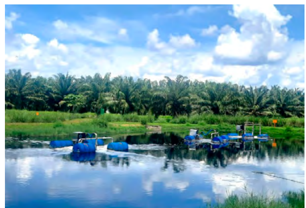
Further aerating the ponds contribute to a better aerobic digestion in our ponds
